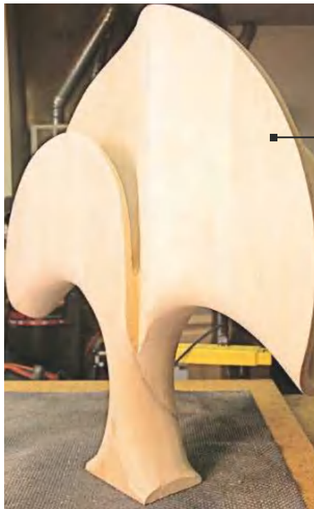
STEP 3. After the cut-out, I shaped the piece with large rotating burrs, hand-held rasps, files and abrasives to obtain the curves and hollows. The inset photo to the right shows a different profile of the shaped piece
